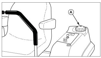
Figure 19. Adding Fuel A. Fuel Cap
